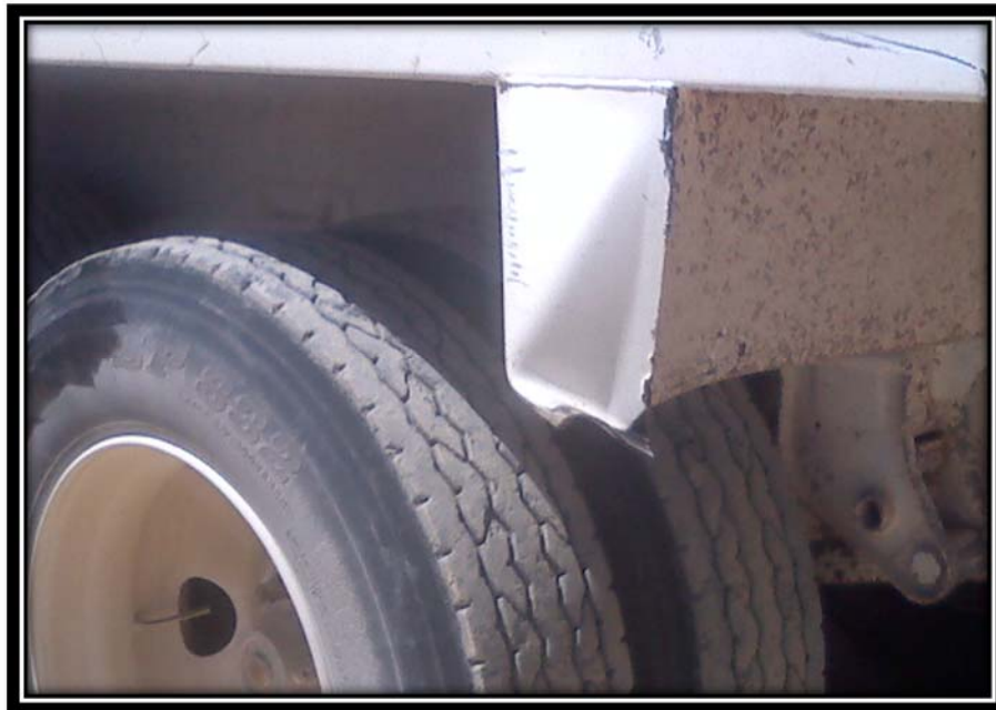
Figure 1: Photograph of damage to the lateral support member on the water loaded tractor-trailer
