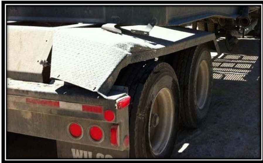
Figure 2: Photograph of damage to right fender of cement loaded tractor-trailer
